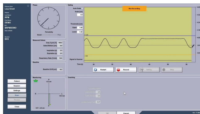
Figure 6 Display of DIBH on the TrueBeam linear accelerator, the level of air in the lungs during free breathing, and by holding the breath in deep inspiration during the delivery of the radiation dose.
